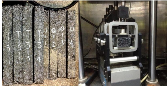
Figure 5. Four-Point Bending Fatigue Test specimen and apparatus
