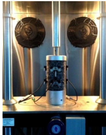
Figure 6. The sample was installed and tested on the SPT machine
