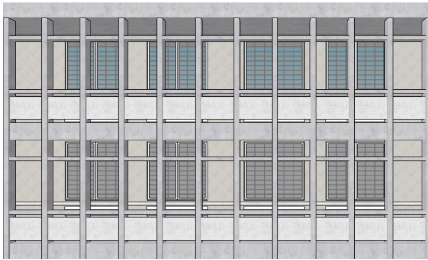
Figure 4. The suspended horizontal beam suggests a purlin within the facade divisions at Ho Chi Minh City University of Architecture, 1976.
