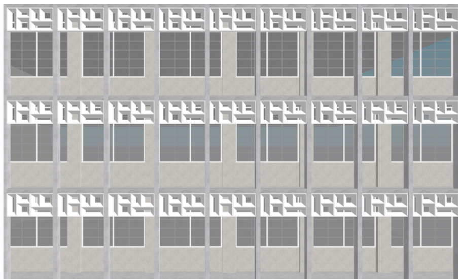
Figure 5. The horizontal division is made of ventilated brick panels attached to the floor beams, forming a decorative feature at Ho Chi Minh City University of Medicine and Pharmacy, 1947.
