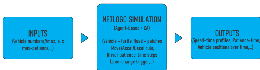
Figure 1. Input–process–output workflow of the NetLogo-based two-lane traffic simulation model
